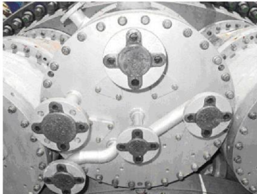
Figure 11. FME Covers On A Combustion Can End-Cover
